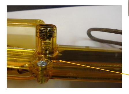
Watch the ball bearing as you are pushing your magazine in to be sure the lip is moving the ball.
